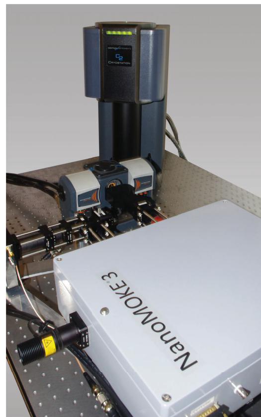
NanoMOKE® 3 incorporated into cryogen-free Montana Instruments Cryostation.
