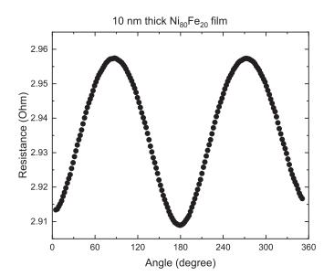
Angular dependence of magnetoresistance measured at 300 K and 1 T using the Resistivity Option in conjunction with the Horizontal Rotator. The 10 nm thick Permalloy film exhibits the expected anisotropic magnetoresistance (AMR) response.
