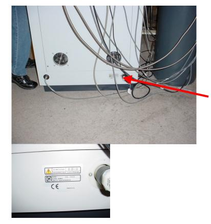
For the MPMS XL, the serial number is located on the bottom rear near the incoming power.
