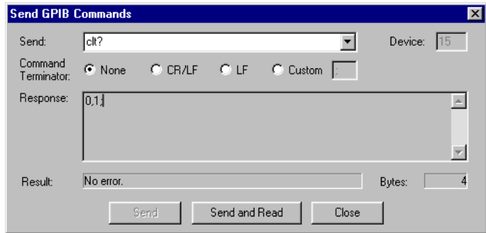
Figure 2. Using the Send GPIB Command dialog to verify control mode
