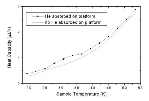
Even with the charcoal holder installed, helium can condense on the sample if the sample is kept below 10 K for several hours. Condensation is especially possible on porous samples, because such samples are very good cryopumps. In this case, cycling the PPMS up to 20 K will flush out the condensed helium.
