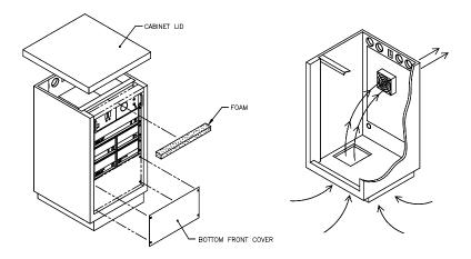
The driver creates an airflow that draws fresh air from the source and pulls it out of the cabinet. The console units are rack mounted and allow the air to flow through the electronics within the console units, thereby exhausting any heat that accumulates within them. With all the heat sources within the cabinet in the path of the airflow, their heat will be drawn out of the cabinet before it has a chance to accumulate and cause the
