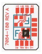
Hall sensor mounted on circuit board
