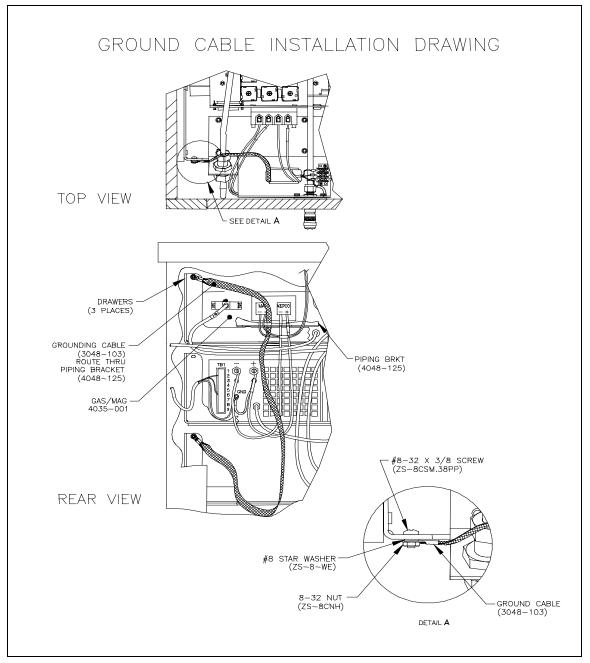
Figure 1. Ground Cable Installation Drawing
