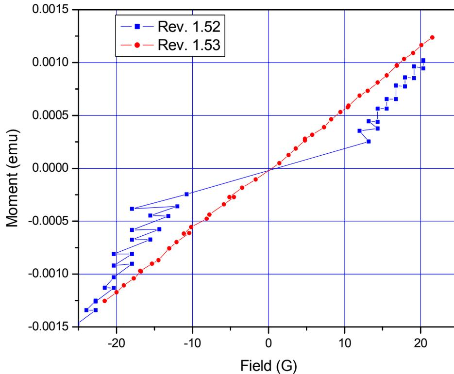
Figure 2. Hysteresis loops for  $\text{Dy}_2\text{O}_3$  sample at 100 K.
