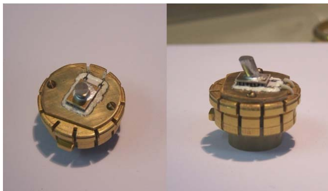
Figure 1– left: top view of the puck with the Peltier element mounted over a brass plate. This plate also holds the heat shield in place; right: lateral view showing a single crystal glued with silver paint. The low temperature epoxy (in white) was applied just on the border of the Peltier element plate to mechanically hold it in place. The thermal contact is provided by a layer of Apiezon N grease previously applied to the Peltier element lower plate.
