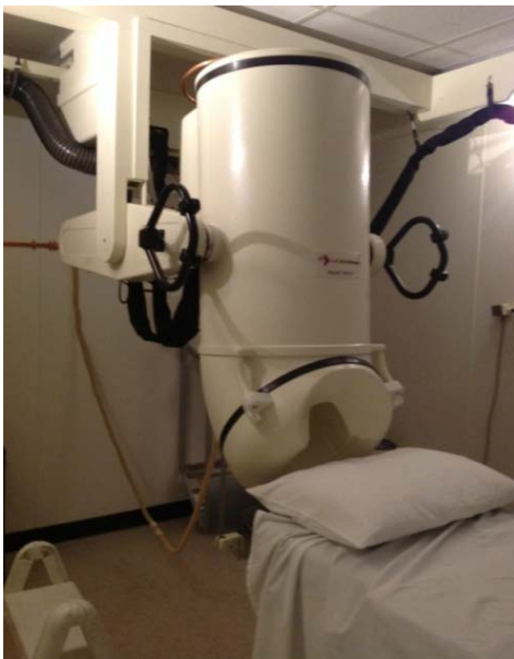
Figure 1. The MEG system installed on a H-frame gantry for translational movement and rotation.
