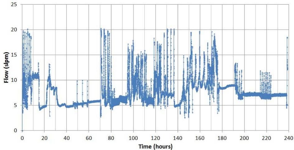
**Figure 2. Typical total flow of Helium boiling off of the instruments (MPMS-XL, PPMS-9T and PPMS-14T) during a period of 10 days of continuous operation. Peaks in the flow are mostly associated with measurements performed at high magnetic fields and changes of sample temperature, which increase helium boil-off. The integrated flow over this 10 day period is 110152 liters of gas, equivalent to 157 liters liquid recovered from the instruments.**
