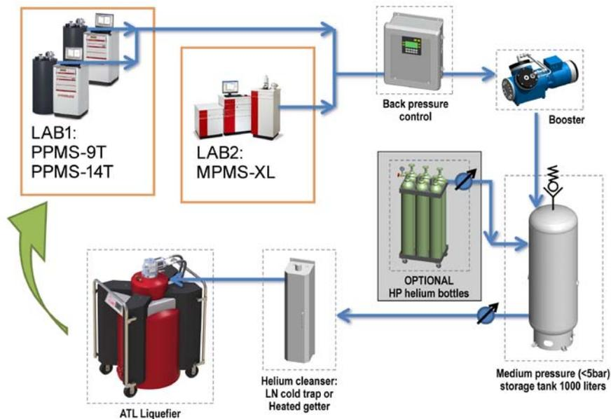
Figure 1. MP-HRP implemented to recover helium boil-off from PPMS and MPMS instruments.
