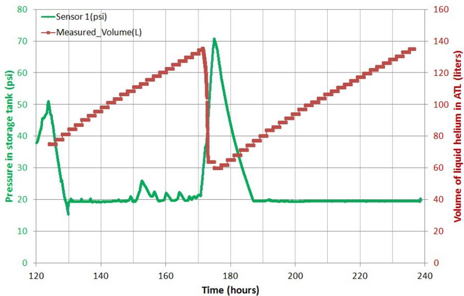
**Figure 3. Pressure in the MP storage tank and liquid level in ATL for the last 5 days of the time interval shown in figure 1. All the helium from the instruments is stored, causing the pressure storage tank pressure to increase, particularly when the liquefaction of ATL is interrupted for a liquid transfer back into the instruments (e.g., at time = 170 hours when 70 liters were transferred from the ATL).**
